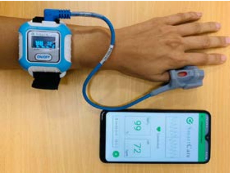
Photo: Wearable pulse oximeter device and smartphone display used for remote monitoring. Figure appeared in: Nguyen Van Vinh Chau, Ho Bich Hai, Greeff Heloise et al. Wearable remote monitoring for patients with COVID-19 in low-resource settings: case study [Internet]. BMJ Innovations. 2021. Available from: http://dx.doi.org/10.1136/bmjinnov-2021-000706
