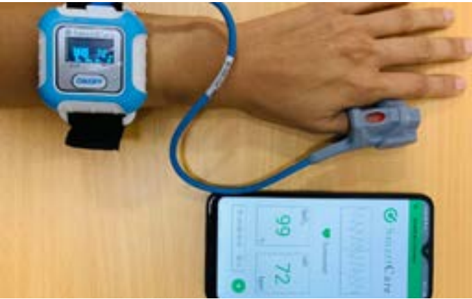
Photo: Wearable pulse oximeter device and smartphone display used for remote monitoring. Figure appeared in: Nguyen Van Vinh Chau, Ho Bich Hai, Greeff Heloise et al. Wearable remote monitoring for patients with COVID-19 in low-resource settings: case study [Internet]. BMJ Innovations. 2021. Available from: http://dx.doi.org/10.1136/bmjinnov-2021-000706
